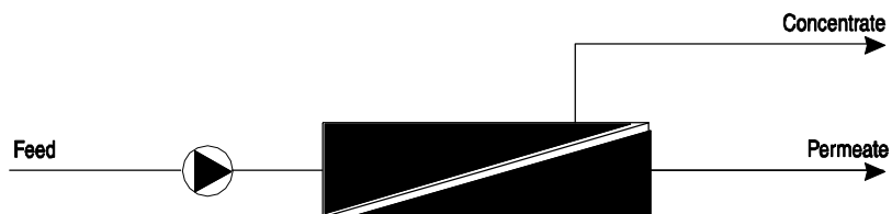
Figure 3.1 Continuous RO process
