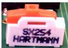
Switch position left (delivery status)
