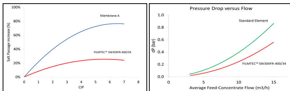
Figure 1: Salt Passage Increase versus number of CIP for SW30XFR-400/34 and Membrane A Figure 2: Element differential pressure versus flowrate for SW30XFR-400/34 and Standard Element
