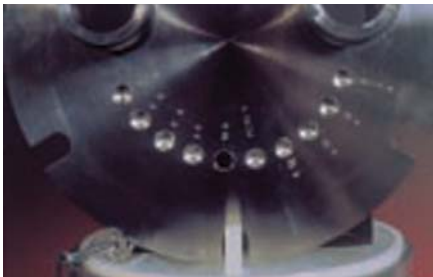
Picture 3: Locating holes with locating pin
